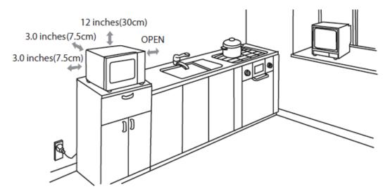
A minimum clearance of 3.0 inches (7.5cm) is required between the oven and any adjacent walls. One side must be open. Leave a minimum clearance of 12 inches (30cm) above the oven.
