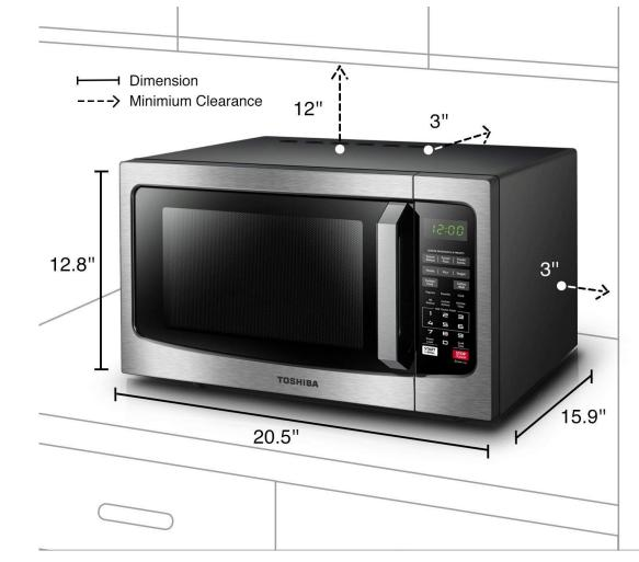
A minimum clearance of 3.0 inches (7.5cm) is required between the oven and any adjacent walls. One side must be open. Leave a minimum clearance of 12 inches (30cm) above the oven.
