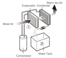
Indoor air passes through the evaporator coils and condenses on the cold coil into water droplets.
