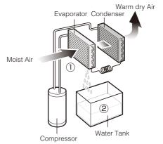
Indoor air passes through the evaporator coils and condenses on the cold coil into water droplets.
