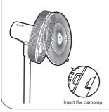
Press the mesh enclosure by both hands in sequence, and when you hear a "click", the installation is in place.
