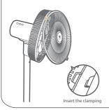
Press the mesh enclosure by both hands in sequence, and when you hear a "click", the installation is in place.
