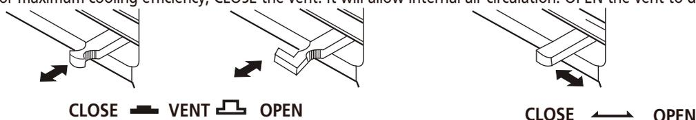
**NOTE: The vent control is not available for all the units. Some units do not have vent control.**
