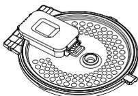
Hold the steam valve and open the small buckle.
