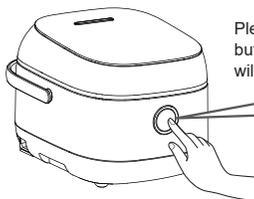
Please do not press the upper housing from above. You should just press the button before hearing the "clatter" sound of unlocking, and the upper housing will be opened.
