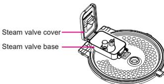
Hold the steam valve and open the small buckle.
