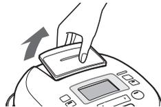
Pull the steam vent upward.
