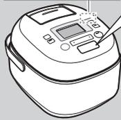
**Vacuum is released with the first pressing of the open button, and the second pressing opens the outer lid.**
