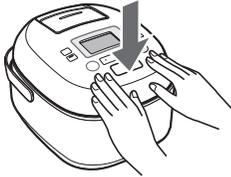
• **The outer lid cannot be closed when the inner lid is not attached.**
