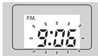
**2** Adjust the hour with the Hrs button and adjust the minute with the Min button.
