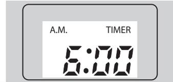
**2** Set the hour with the **Hrs** button and set the minute with the **Min** button.
