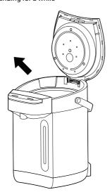
**2** Turn on the power supply and boil the descaling agent solution
