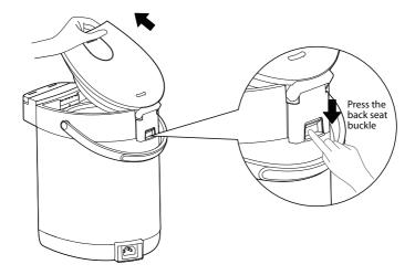
2 Installing the lid: Press the back seat buckle with one hand, align the lid with the connecting shaft with the other hand, place it in the slot, and then release the back seat buckle to fix the lid and complete the lid installation
