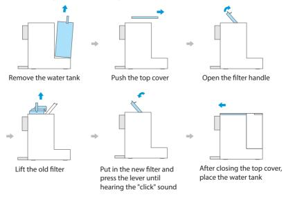
②After replacing the filter, hold the Filter Reset button for 3 seconds to reset the filter life.
