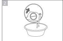
2. In case of power failure, open the filter door to drain the cooled water in the drum.
