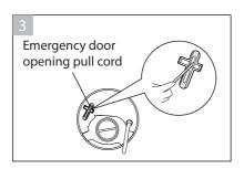
Insert the tool into the pull ring and pull it downward to unlock the door of the machine
