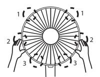
**3** Fix the clip using screw after locking.
