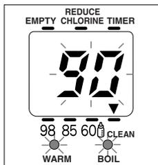
► The WARM and BOIL indicators will flash. The remained time of the cleaning will flash in the display of minutes.
