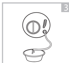
3 After water runs out, reset the drain hose
