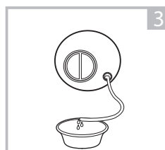
After water runs out, reset the drain hose
