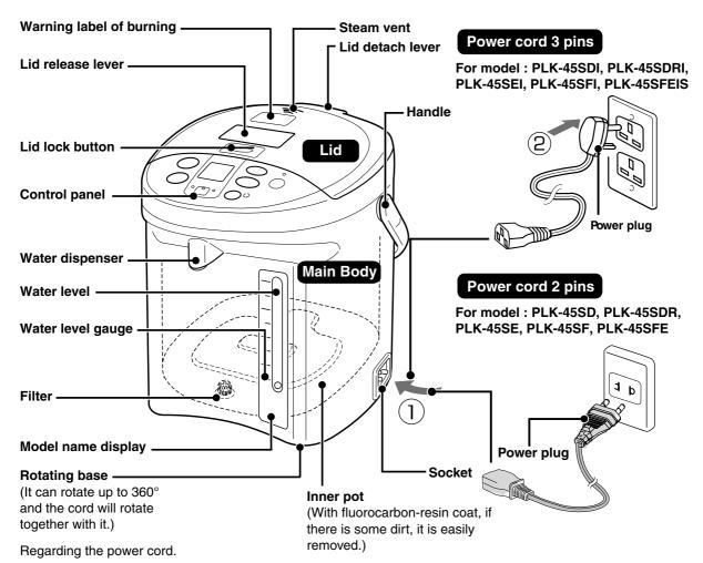
For the figure, the power cord 3 pins plug is for grounded socket version.
